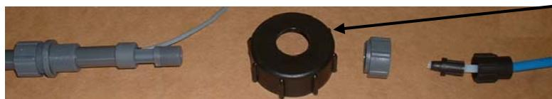
Tightening cap allowing adjustment of tube insertion depth
