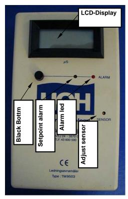
The purpose of the conductivity meter is to measure and show the conductivity and give alarm signal in case of excess of set value or power failure.
