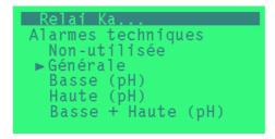
The general technical alarm only concerns physical faults in the sensors or electronics, and do not concern the programmable alarm threshold values.
