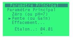
Thus, for a pH probe, a standard value of 4.01 was validated. However, the user can easily change this reference and use that shown on the measurement electrode (example: pH=9.21)
