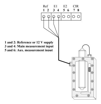
The wires on the  $PROBOX^{\otimes}$  measurement chamber are colour coded as a function of the type of sensor used.
