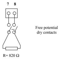
The resistor can be installed remotely, there is no limit on cable length.
