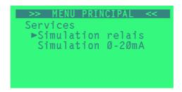
Immediately following the exit from the « Services » function, the relays that have been set or the 0...20 mA outputs that have been programmed, are automatically reset to « 0 ».
