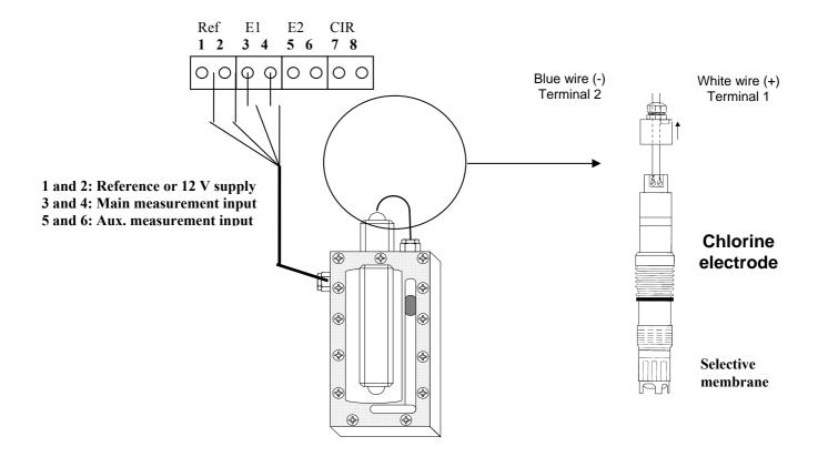
The wires on the  $PROBOX^{\otimes}$  measurement chamber are colour coded as a function of the type of sensor used.
