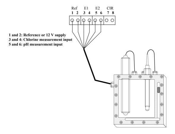
The wires on the  $PROBOX^{\otimes}$  measurement chamber are colour coded as a function of the type of sensor used.
