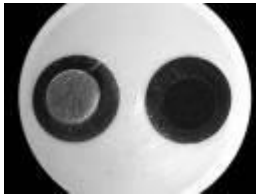
Electrodes oxidised after four months of operation
