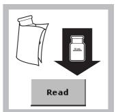
**12.** Wipe the prepared sample and insert it into the cell holder with the fill line facing right.
