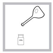
9. Prepared Sample: Pour 10 mL from the second volumetric flask into a second sample cell.
