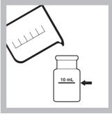
**3. Blank Preparation:** Fill a square sample cell with 10 mL of sample and stopper.
