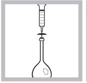
3. Blank Preparation: Using the syringe and needle provided, add 1.0 mL of Chlorine Dioxide Reagent A into a 25-mL volumetric flask.
