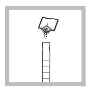
5. Blank Preparation: Add the contents of one Dechlorinating Reagent Powder Pillow to one cylinder. (This is the blank).
