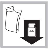
**10.** Within one minute of adding the DPD reagent, wipe the sample cell and insert it into the cell holder with the fill line facing right.
