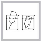
**6.** Fill a DPD Free Chlorine Reagent AccuVac Ampul with sample. Keep the tip immersed while the Ampul fills completely.
