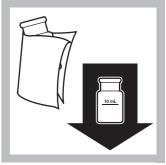
**4.** Wipe the blank and insert it into the cell holder with the fill line facing right.
