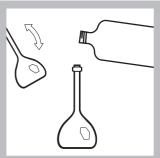
**4.** Fill the volumetric flask to the mark with deionized water. Stopper. Invert at least 7 times to mix.
