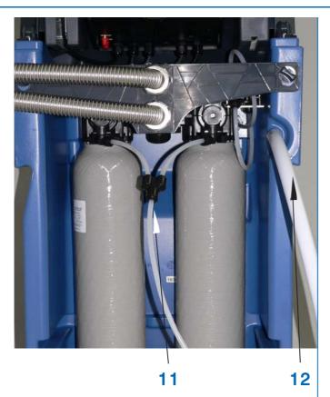
Attach the rinsing water hose (11) firmly to the Y piece.
