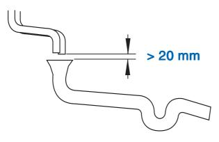
Please note: According to EN 1717 the rinsewater and overflow hoses must be attached with at least a 20mm clearance of the highest possible waste-water level at the drain (free outflow).
