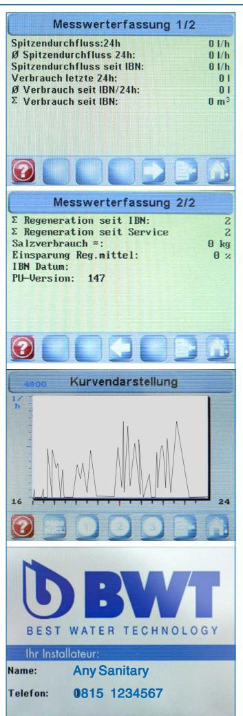
Data acquisition displays the consumption values for water and regenerants.
