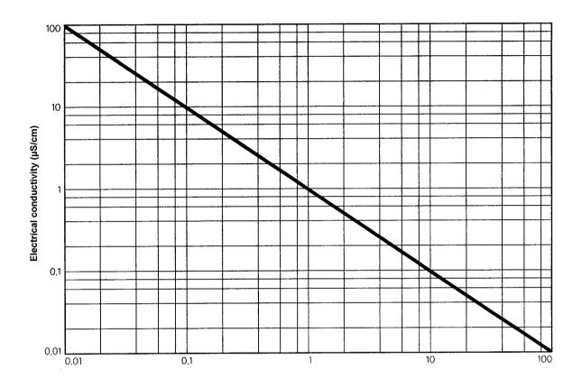
Electrical resistance (10<sup>6</sup>  $\Omega$ .cm = M $\Omega$ .cm)
